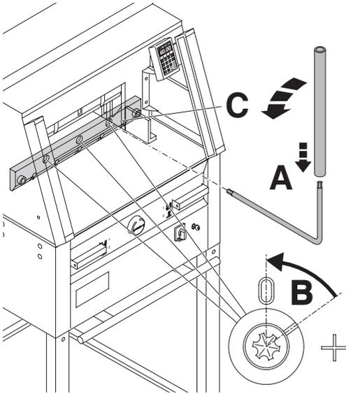
The 3 eccentrics are now exposed and should be turned counter clockwise to position "0" with the special wrench and attachable extension pipe (A) (in the tool set). The slot must correspond to position "0" (B).
