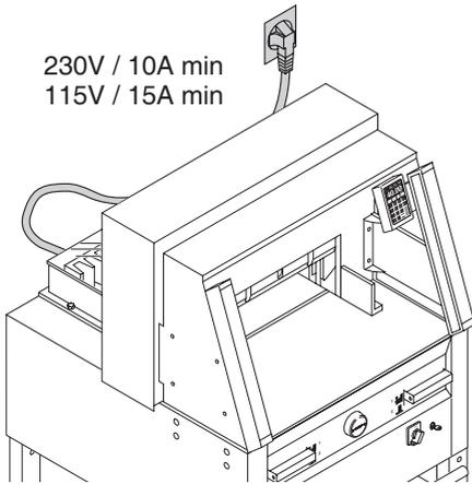
Connect the power cord to a single phase socket.
