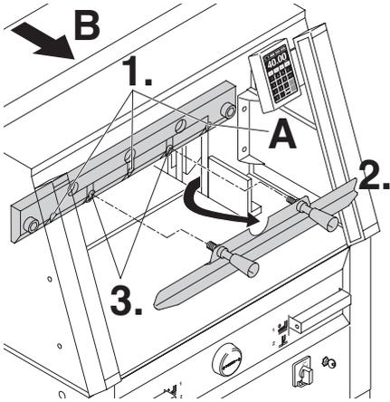
Lightly tighten 3 (4860 has 2) of the 5 blade screws with washers (1.). Remove the blade changing tool (2.). Lightly tighten the remaining blade screws with washers (3.). Return blade changing tool to tool holder (B).
