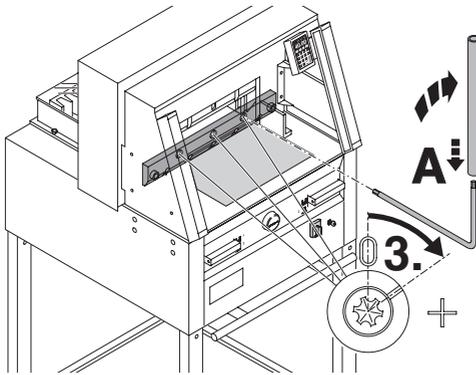
With the special wrench (A) the 3 eccentrics should be screwed down (3.) until the paper is cut along the entire length of the blade (The blade must remain parallel, not too deep into cutting stick).
