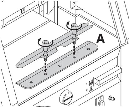
Take the exchange blade carefully out of the blade box and screw it to the blade changing tool (A).
