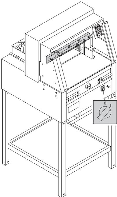
Remove the special wrench and turn on the main switch until the blade returns to the home position.
