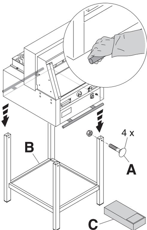
4 strong people are required to lift the machine from the pallet and place it on the stand. Secure with 4 screws (**A**). Put the shelf (**B**) on the stand. (Parts and tools are in the tool set) (**C**).
