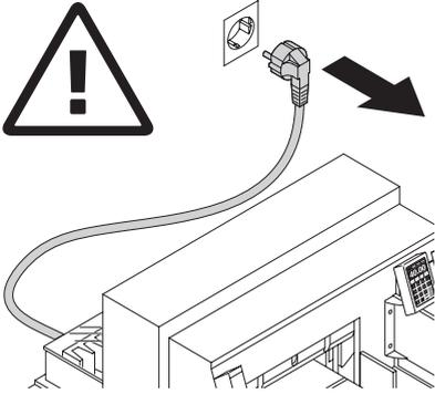
**⚠ Danger! Disconnect the mains before starting any service work or before removing the cover.**
