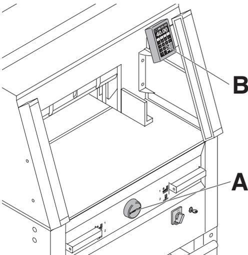
The measurement is set either with the hand-wheel (A) or by programming (B) the cutting measurements. Measurement is shown on the display in inches or cm (B).
