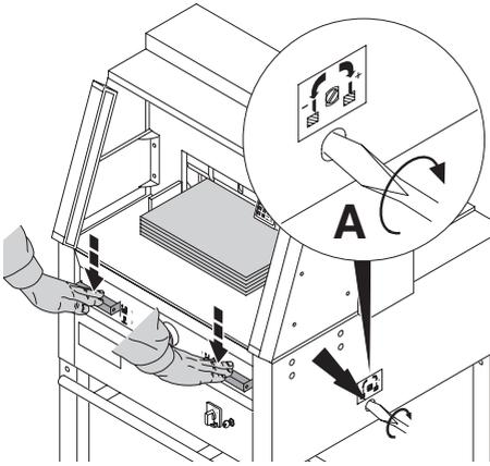
Paper cutting test. If the last sheet or several sheets are not completely cut, gradually turn the knob for blade depth adjustment (A)  $\frac{1}{4}$  turn to the right until the paper is cut along the entire length. Do not set too low as blade will become blunt sooner.
