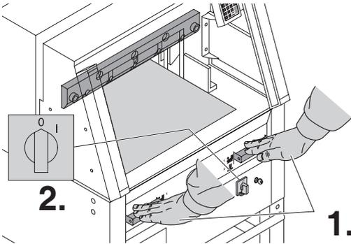
Lower the blade by pressing both cutting buttons (1.). Keep one button pressed and turn off the main switch (2.).
