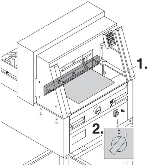
Remove all tools and distribute paper along the entire cutting length (1.). Turn main switch to position "I" (2.).
