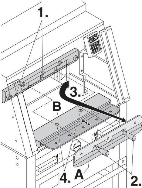
Remove 2 blade screws 4860 and 3 blade screws 5260, 6660 (1.).
