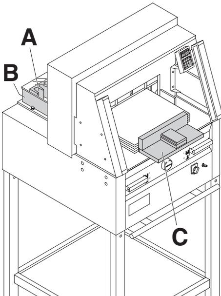
Position the paper on the backgauge (A) and side lays left or right (B). To move paper stacks, please use the paper knock-up block (C) provided. (Run backgauge to the front for turning the paper stack).
