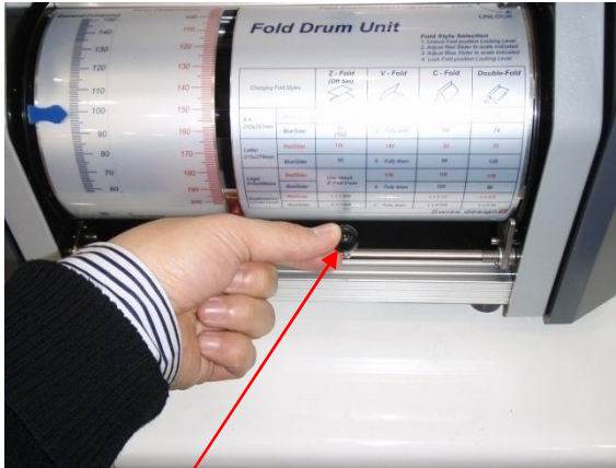
Folding Drum handle in the Unlock(down) position
