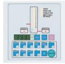
Programming and operation is controlled from an easy-to-use touch-button control panel.
