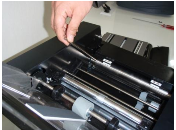
[Insert the jam removal onto the hole of roller and pull it down ]
