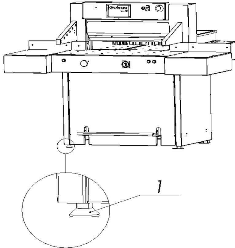
Drawing 2. Adjustment of cutter positioning
