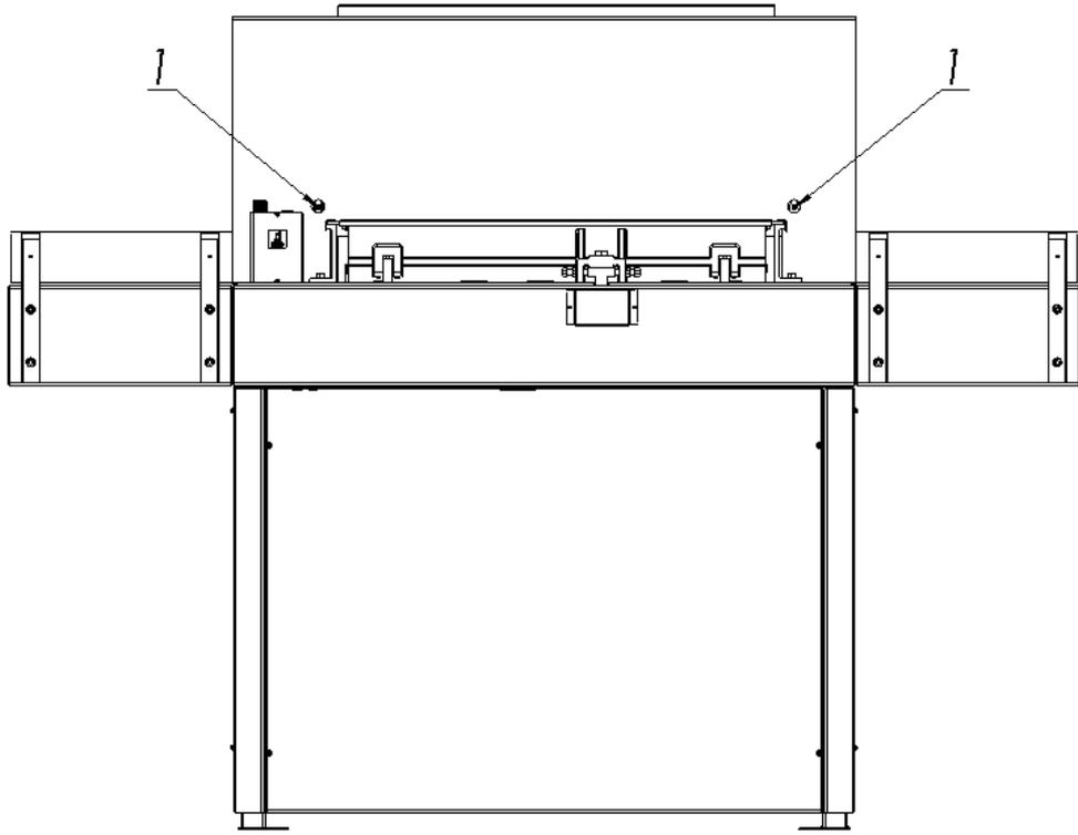
Drawing 40 Clamp bar lubrication points location
