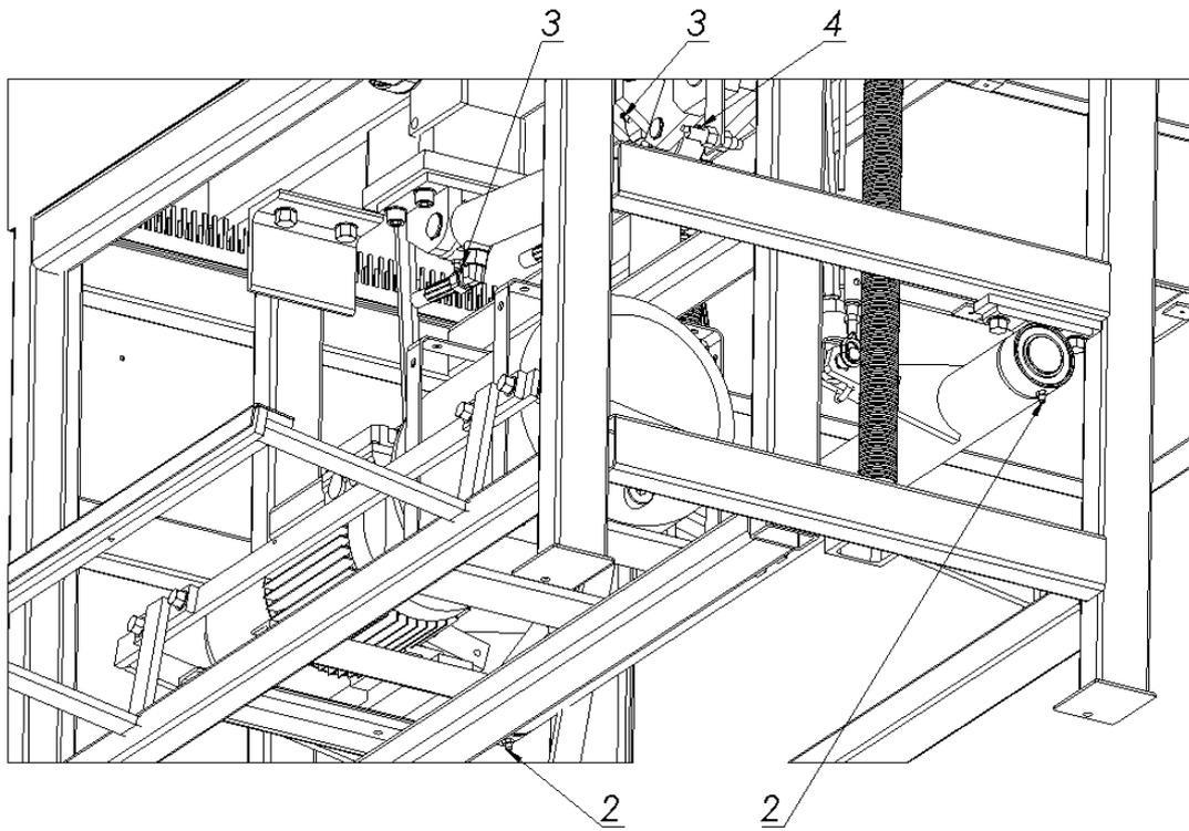
Drawing 41. Roller bearing 2, hydraulic actuators fixing 3, knife band head 4.
