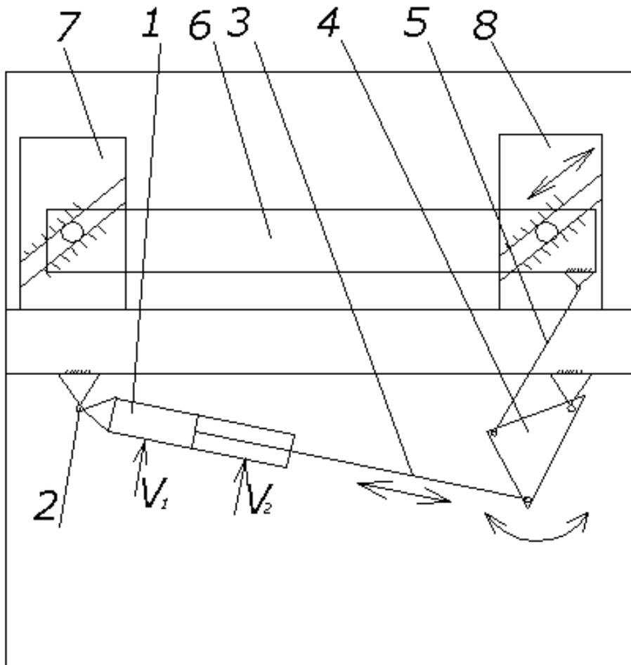
Drawing 4. Kinematic diagram of the knife driving mechanism
