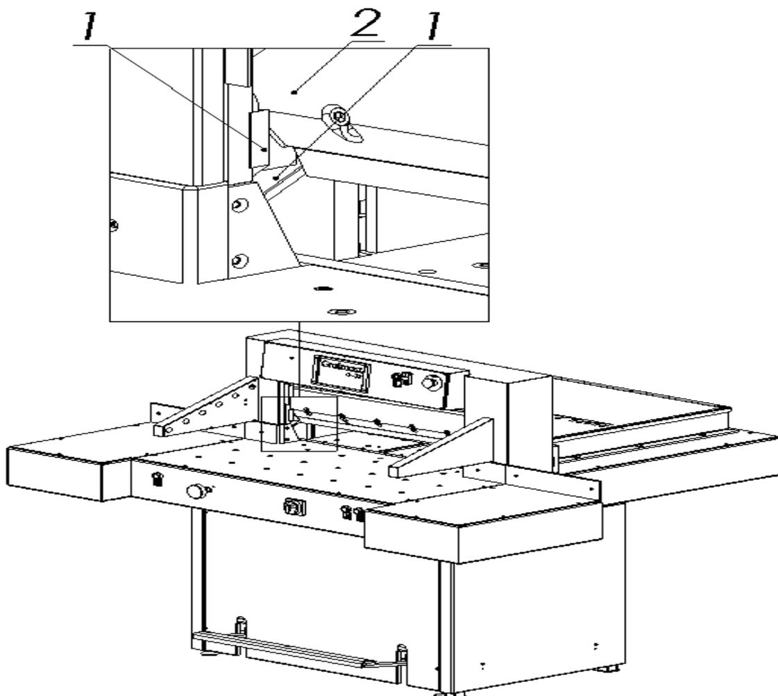
Drawing 37 Locations of the knife lubrication locations (knife in Upper position)
