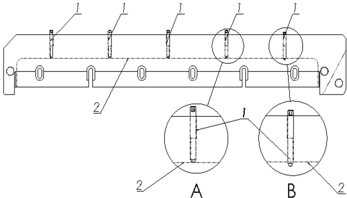
Drawing 21. Adjusting screws position.
