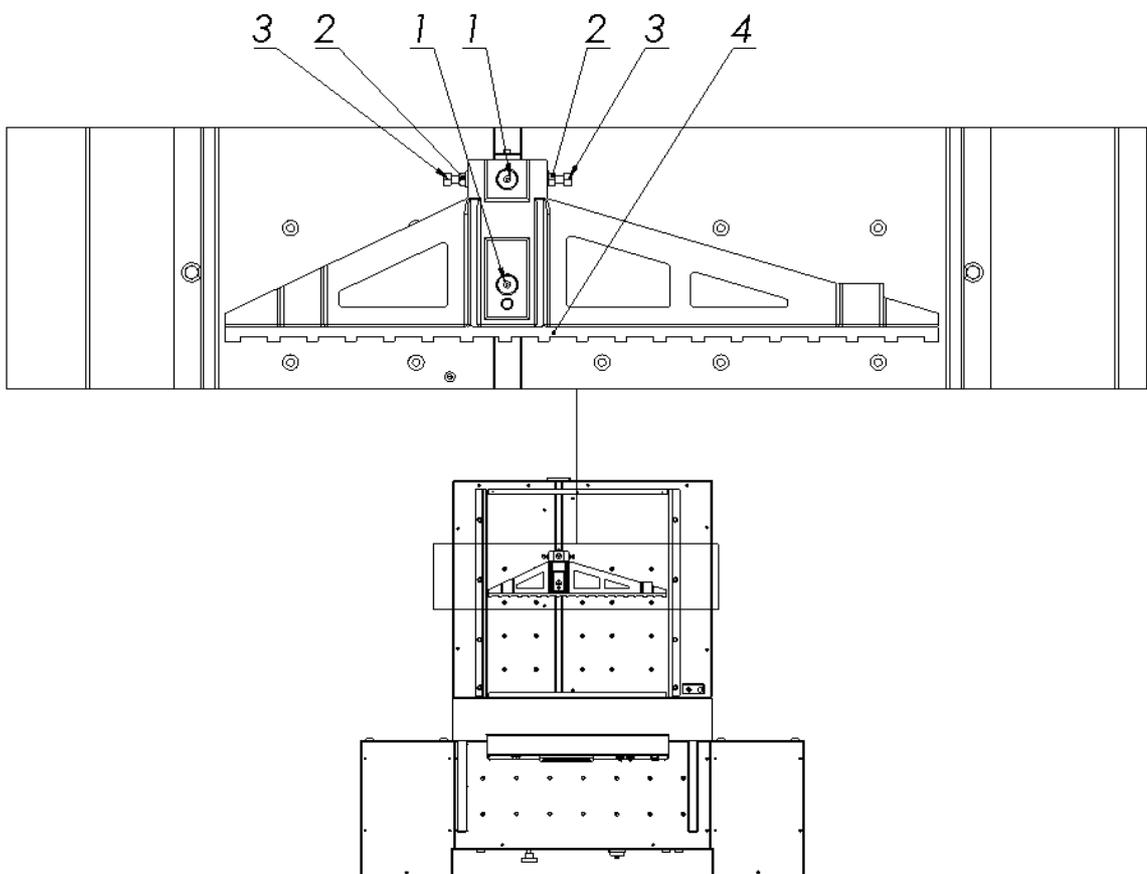
Drawing 31 Backgauge parallelism adjustment
