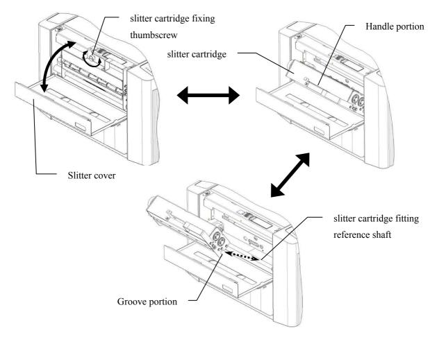
\* Make sure to engage gears of slitter cartridge and machine each other.
