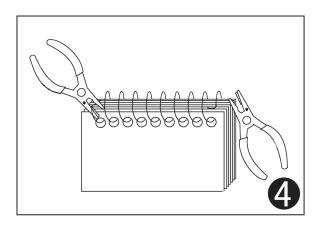
Upon completion of coil insertion, be sure to put the crimper back in the Coil Crimper Holder.
