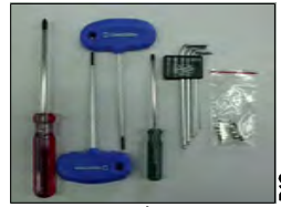
Maintenance tools: 1. Cross-head and flat-head screwdriver - each 1 pc 2. T-type hex wrench (2.5,3) - each 1 pc 3. Hex wrench (1.5/2/2.5/3/4) - each 1 pc 4. Fuse (7A) - 5 pcs
