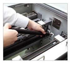
**EASY MAINTENANCE** The Prime now has detachable rollers, not only making cleaning easy, but it gives better access to components in case of a paper jam.
