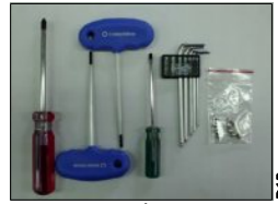
Maintenance tools: 1. Cross-head and flat-head screwdriver - each 1 pc 2. T-type hex wrench (2.5,3) - each 1 pc 3. Hex wrench (1.5/2/2.5/3/4) - each 1 pc 4. Fuse (4A) - 5 pcs
