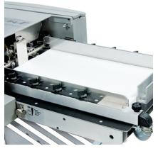
**TOP-LOADING PAPER FEED** A top-loading paper feed system allows continuous operation.
